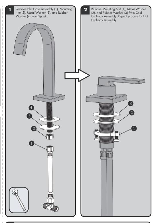
Place Spout Assembly through the center hole of counter top. From below, reinstall the Spout 5 Rubber Washer (1), Metal Washer (2), and Mounting Nut (3). Loosely assemble at this time. Reinstall Inlet Hose Assembly (4)
