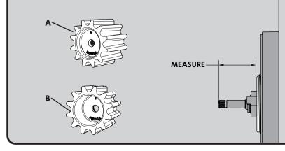
Confirm that the Valve is in the off position. Insert Spline Adapter 🕕 (Spline Adapter selection determined in STEP 3) over Valve Spindle 2. One set of splines on the adapter must be oriented perfectly vertical when installed, as shown below. Secure the Spline Adapter with the 8-32 X 3/8" Screw 3 provided.
