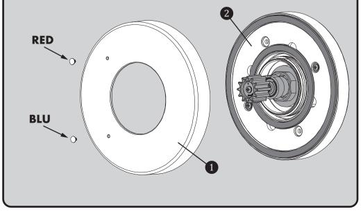
Orient the Handle Assembly in a vertical position as shown below. Guide Handle Assembly onto the Spline Adapter (3). While holding the Handle (1) stationary in the vertical position, thread the Handle Escutcheon (2) onto the Wall Mounting Plate (4). Hand tighten until snug.
