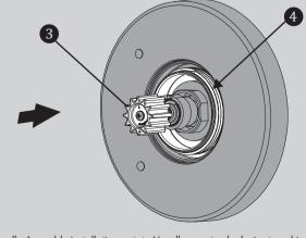
**NOTE:** After Handle Assembly installation, rotate Handle counterclockwise to achieve full closure of Valve. If the Handle does not rest in a vertical position, repeat Steps 9 and 11 for proper Handle alignment.
