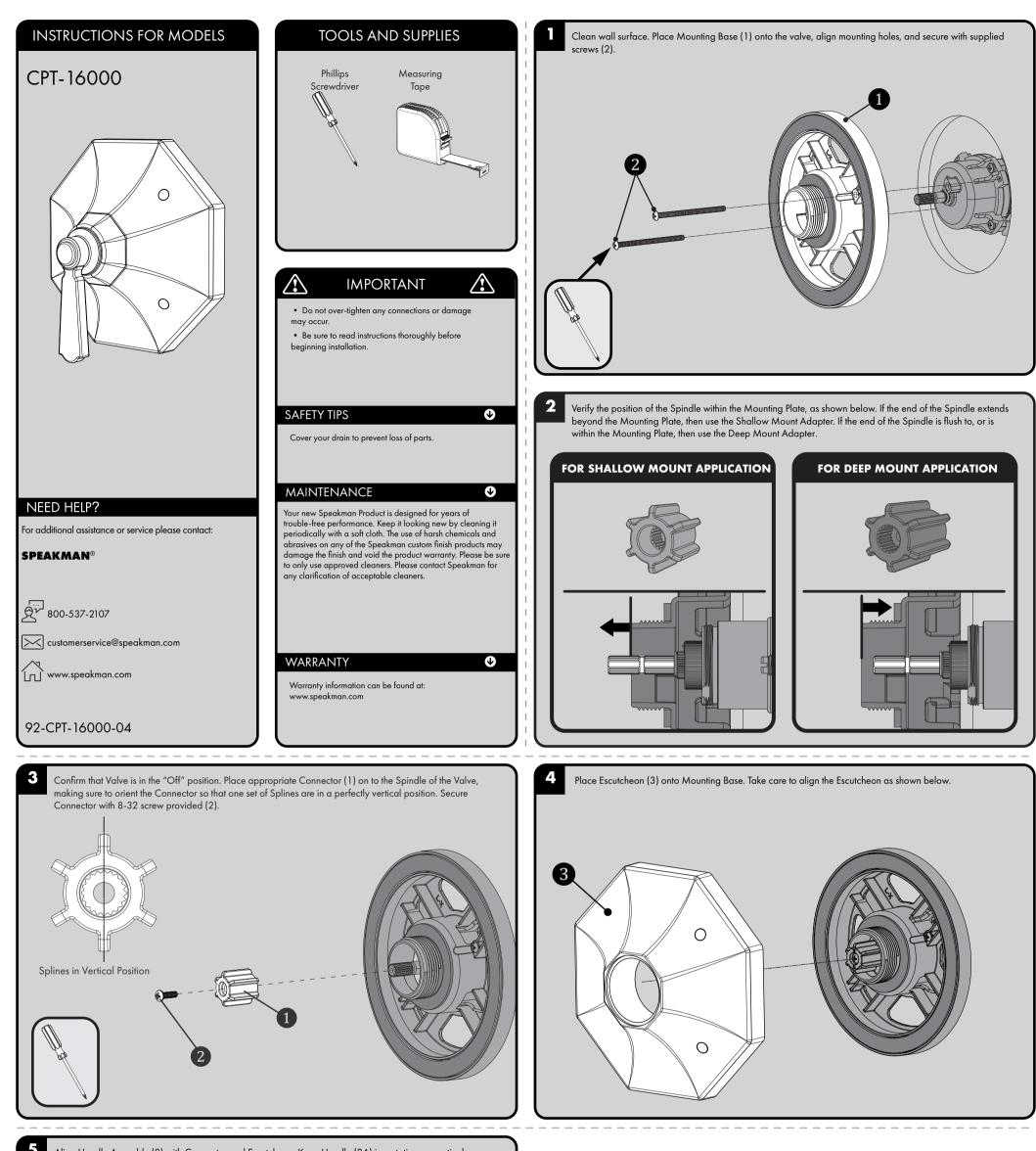
Align Handle Assembly (8) with Connector and Escutcheon. Keep Handle (8A) in a stationary vertical
