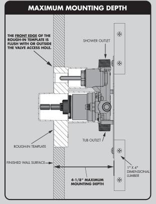
Mounting Structure behind the wall must be capable of supporting the Valve in use. Following the rough-in dimensions for your model of valve (located ot the end of this manual), reference the diagram below for the installation and placement of the bracing within a 2"x4" wall, using a 1"x4" brace. Mounting hardware is not included.
