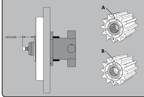
Confirm that the Valve is in the off position. Insert Spline Adapter (1) over Kohler spindle (2), with the appropriate side "A" or "B" facing outward. (determined in Step 4). One set of splines on the adapter must be oriented perfectly vertical when installed, as shown below. Secure the Spline Adapter with the 8-32 X 7/8" Screw (3) provided.
