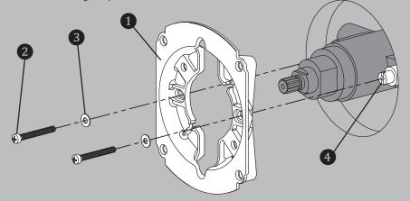
**NOTE:** The back surface of the Valve Mounting Plate Assembly (1) should sit flush against the wall when installed correctly.
