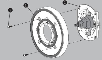
**NOTE:** The back surface of the Valve Mounting Plate Assembly (1) should sit flush against the wall when installed correctly.
