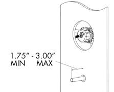
Slide spout (1) over exposed stub out pipe until flush to wall. Center the spout (1) on the wall and tighten set screw (2) from underneath with Allen wrench
