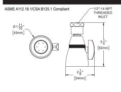
Model: S-2292 Max. Flow Rate: 2.5 gpm (9.5 L/min) Min. Flow Rate: 2.0 gpm (7.6 L/min) @ 45 psi For use with automatic compensating valves rated at 7.6 L/min (2.0 gpm) or less.
