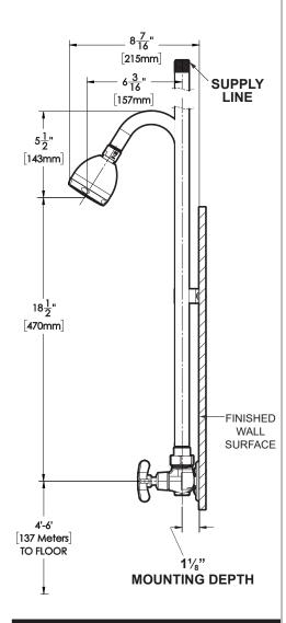
NOTE: Supply lines must have 1/2 NPT female threaded ends and be 1-1/8" from center of supply line to finished wall.
