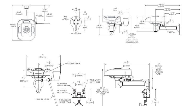
1. All dimensions are in inches (millimeters) unless otherwise specified and are subject to change without notice. 2. This unit should be connected to an uninterrupted source of potable water, with a minimum flowing pressure of 30 psi and a maximum static pressure of 125 psi. 3. Before mounting mixing valve, verify the supply hose will reach the connection.
