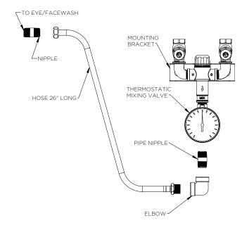
1. All dimensions are in inches (millimeters) unless otherwise specified and are subject to change without notice. 2. Before mounting, verify the supply hose will reach the connection.
