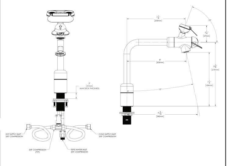
NOTE: UNLESS OTHERWISE SPECIFIED, ALL INLETS ARE 3/8" COMPRESSION WITH FEMALE THREADS. UNLESS OTHERWISE SPECIFIED, ALL DIMENSIONS ARE IN INCHES AND ARE SUBJECT TO CHANGE WITHOUT NOTICE.
