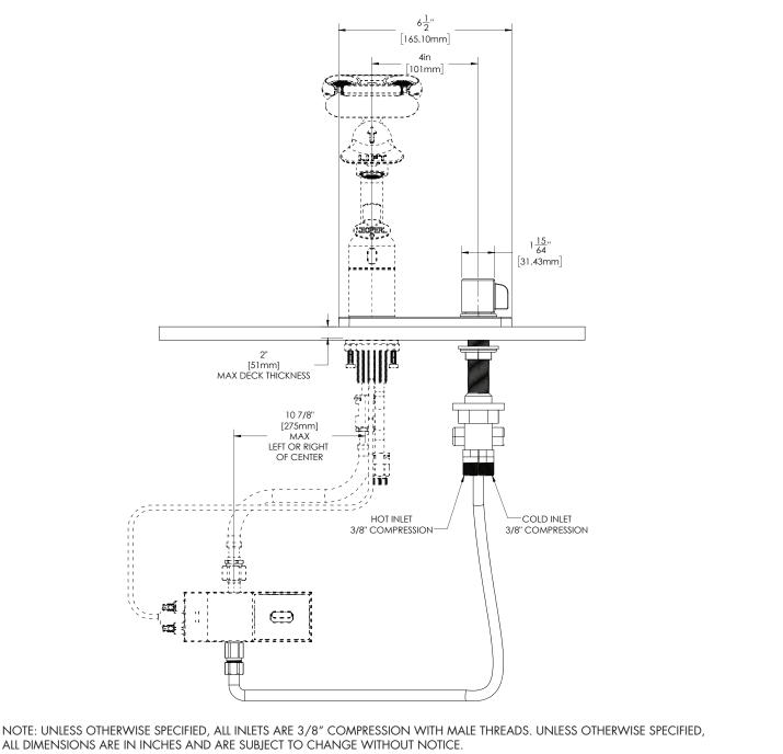
NOTE: UNLESS OTHERWISE SPECIFIED, ALL INLETS ARE 3/8" COMPRESSION WITH MALE THREADS. UNLESS OTHERWISE SPECIFIED,
