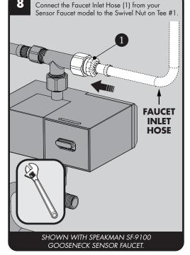
NOTE: Complete Mounting and Electrical Connections of the Solenoid Box following the Installation Manual included with your Sensor Faucet.
