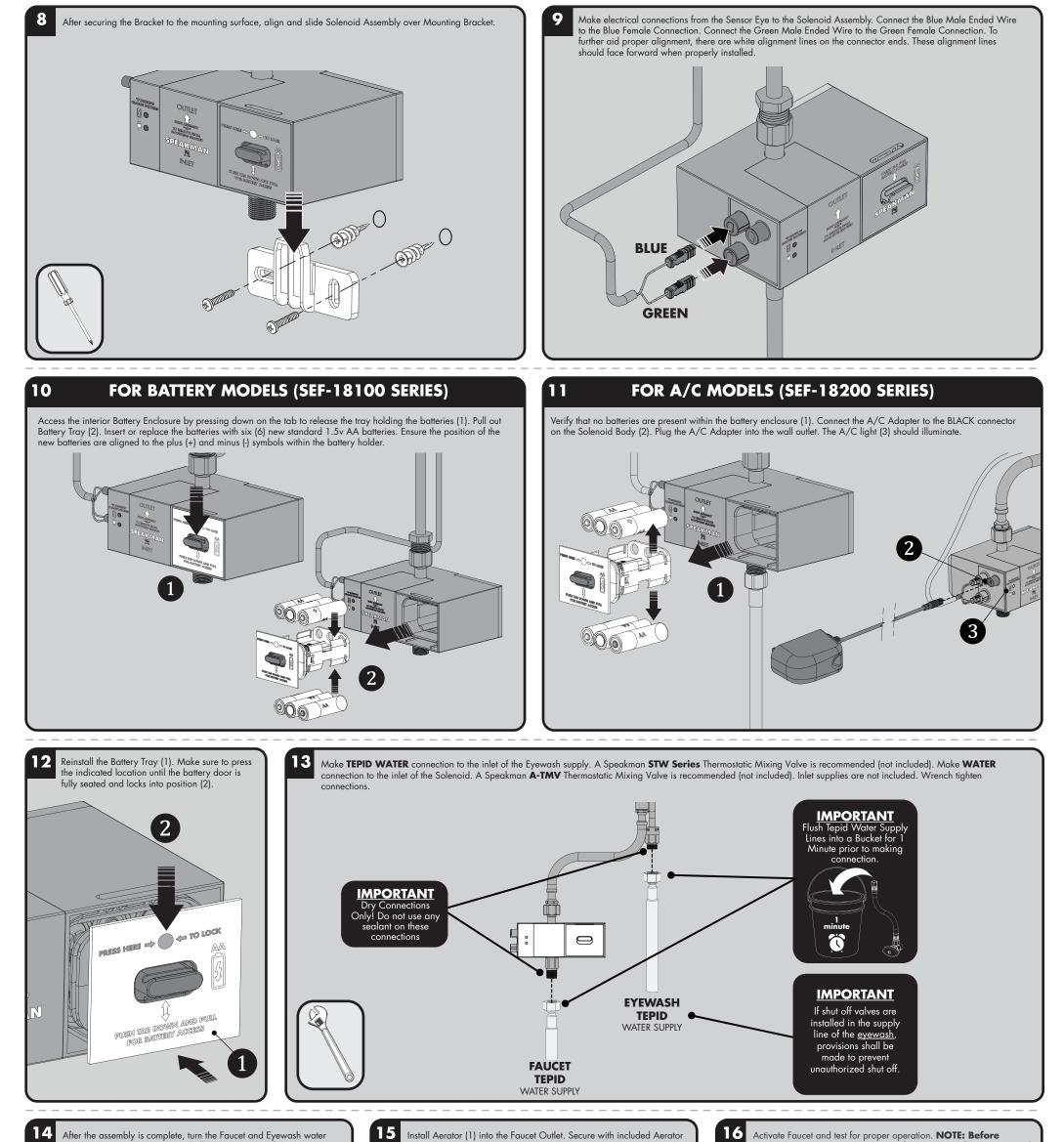
After the assembly is complete, turn the Faucet and Eyewash water supplies on. Activate Sensor and allow Faucet to run for 1 minute to flush out any debris. Check all connections for leaks.
