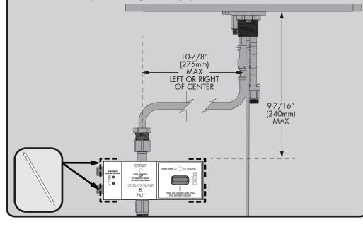
ng Bracket (1) from Solenoid Assembly. Using the previously marked location on m iove Ivio ounting surface, align Mounting Bracket (1) horizontally to approximate position and mark the mounting locations with a pencil. If mounting on drywall and not to stud, use the appropriate anchors and fasteners for application. Recommend screw in easy anchor or equal for drywall.
