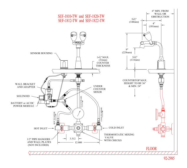
SEF-1810-TW -4" Sensorflow, eyewash faucet, UCM, battery and Thermostatic Valve for Eyewash SEF-1820-TW -4" Sensorflow, eyewash faucet, UCM, AC/DC and Thermostatic Valve for Eyewash SEF-1812-TW -8" Sensorflow, eyewash faucet, UCM, battery and Thermostatic Valve for Eyewash SEF-1822-TW -8" Sensorflow, eyewash faucet, UCM, AC/DC and Thermostatic Valve for Eyewash
