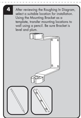
drill holes in marked locations. Insert Wall Anchors into wall and ensure they are flush with the wall surface. Secure Bracket to Wall Anchors with the included Mounting Screws.
