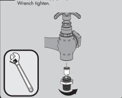
Tighten the Threaded Insert to create a seal between the Sink Fitting and the Adapter using a 5/16" Allen Wrench in the base of the
