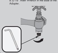
After applying Thread Sealant Tape, thread the Vacuum Breaker Assembly (1) onto the Stop Adapter. Wrench tighten.
