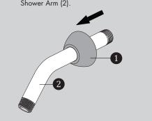
Apply Teflon Tape to inlet side of Shower Arm (2). Thread Shower Arm (2) into Female Pipe Fitting within the wall. Firmly tighten, and make sure Shower Arm (2) Outlet is pointing in a downward position.
