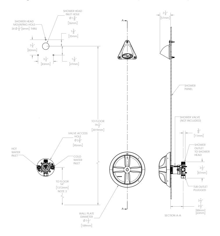
1. All dimensions are in inches (millimeters) unless otherwise specified and are subject to change without notice. 2. Unless otherwise specified all inlets and outlets are 1/2" female copper sweat and 1/2" male NPT. 3. For ADA mounting locations consult ADAAG, ANSI A117.1 or state regulations.
