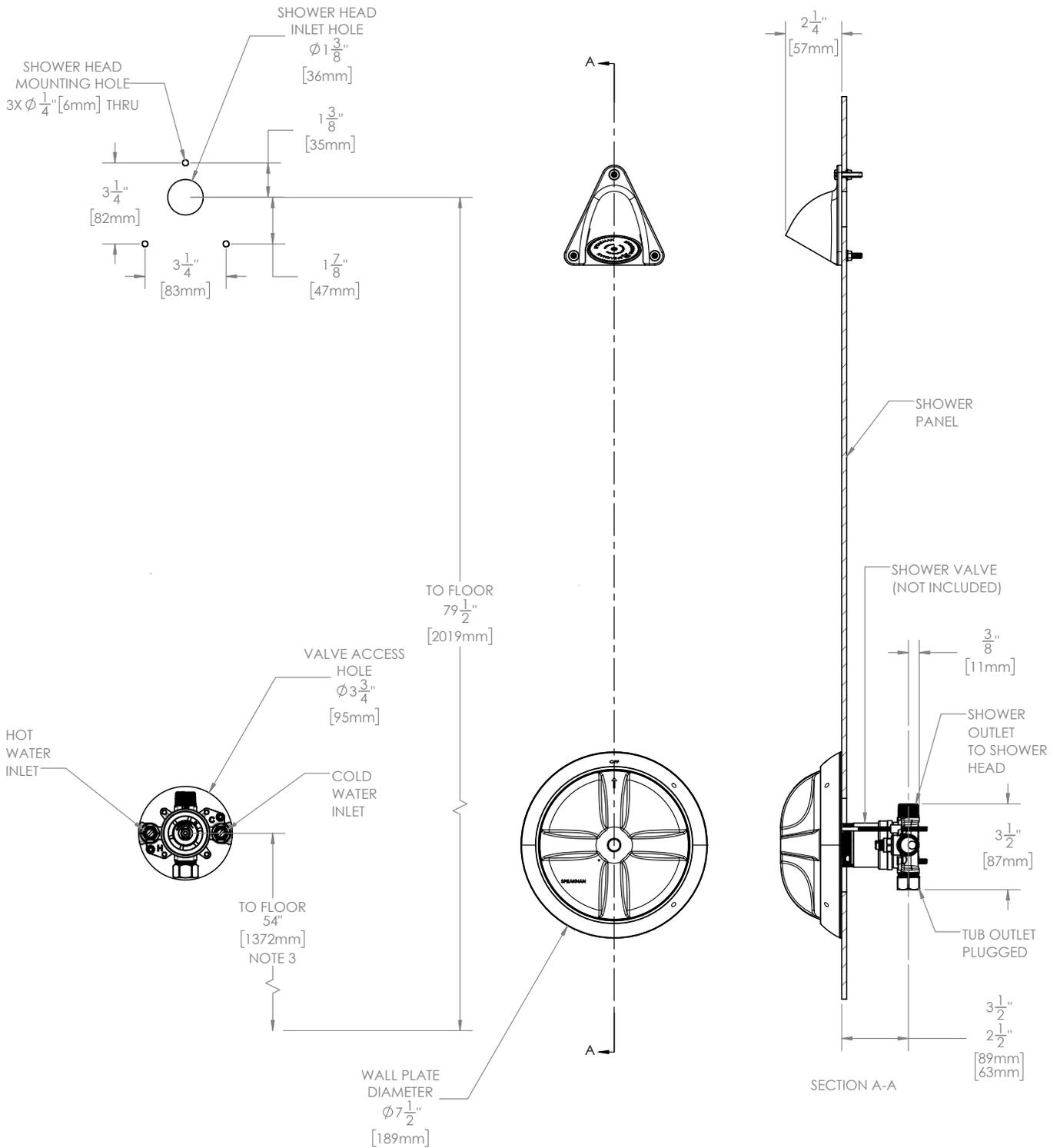
1. All dimensions are in inches (millimeters) unless otherwise specified and are subject to change without notice. 2. Unless otherwise specified all inlets and outlets are 1/2" female copper sweat and 1/2" male NPT. 3. For ADA mounting locations consult ADAAG, ANSI A117.1 or state regulations.
