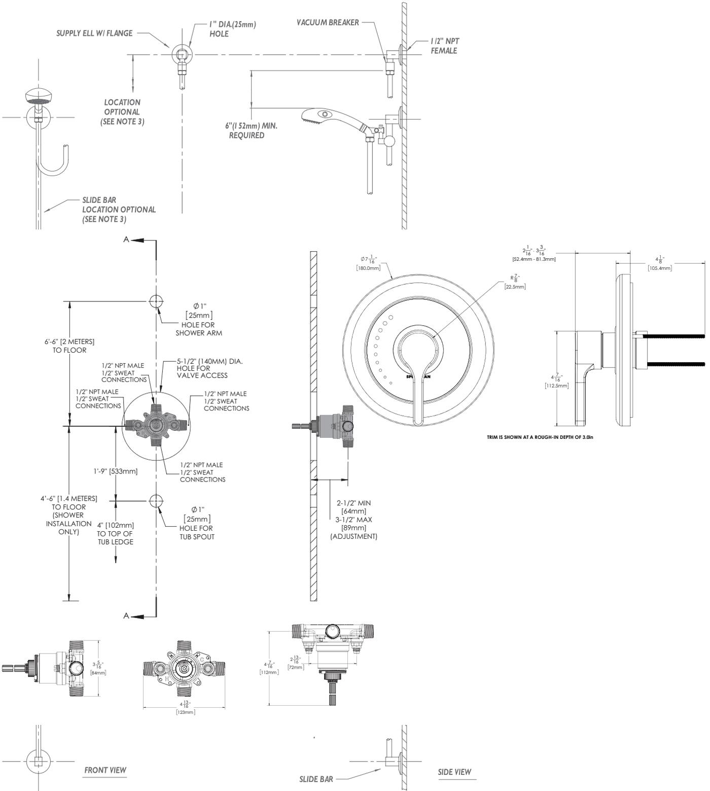
NOTE: 1. All dimensions are in inches (millimeters) unless otherwise specified and are subject to change without notice. 2. Unless otherwise specified, all inlets and outlets are 1/2" female copper sweat. 3. For ADA mounting locations, consult ADAAG, ANSI A117.1, or static regulations
