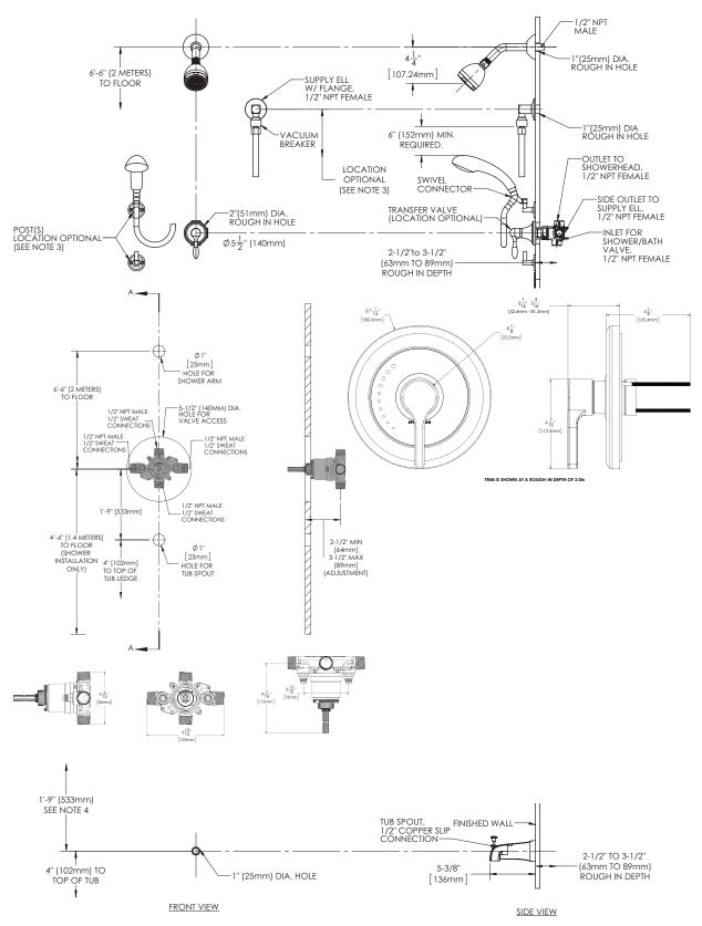
NOTE: 1. All dimensions are in inches (millimeters) unless otherwise specified and are subject to change without notice. 2. Unless otherwise specified, all inlets and outlets are 1/2" female copper sweat. 3. For ADA mounting locations, consult ADAAG, ANSI A117.1, or static regulations
