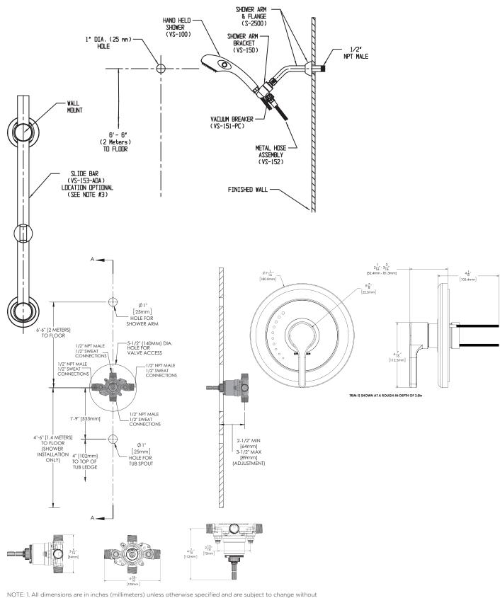
NOTE: 1. All dimensions are in inches (millimeters) unless otherwise specified and are subject to change witho notice. 2. Unless otherwise specified, all inlets and outlets are 1/2" female copper sweat. 3. For ADA mounting locations, consult ADAAG, ANSI A1171, or static regulations
