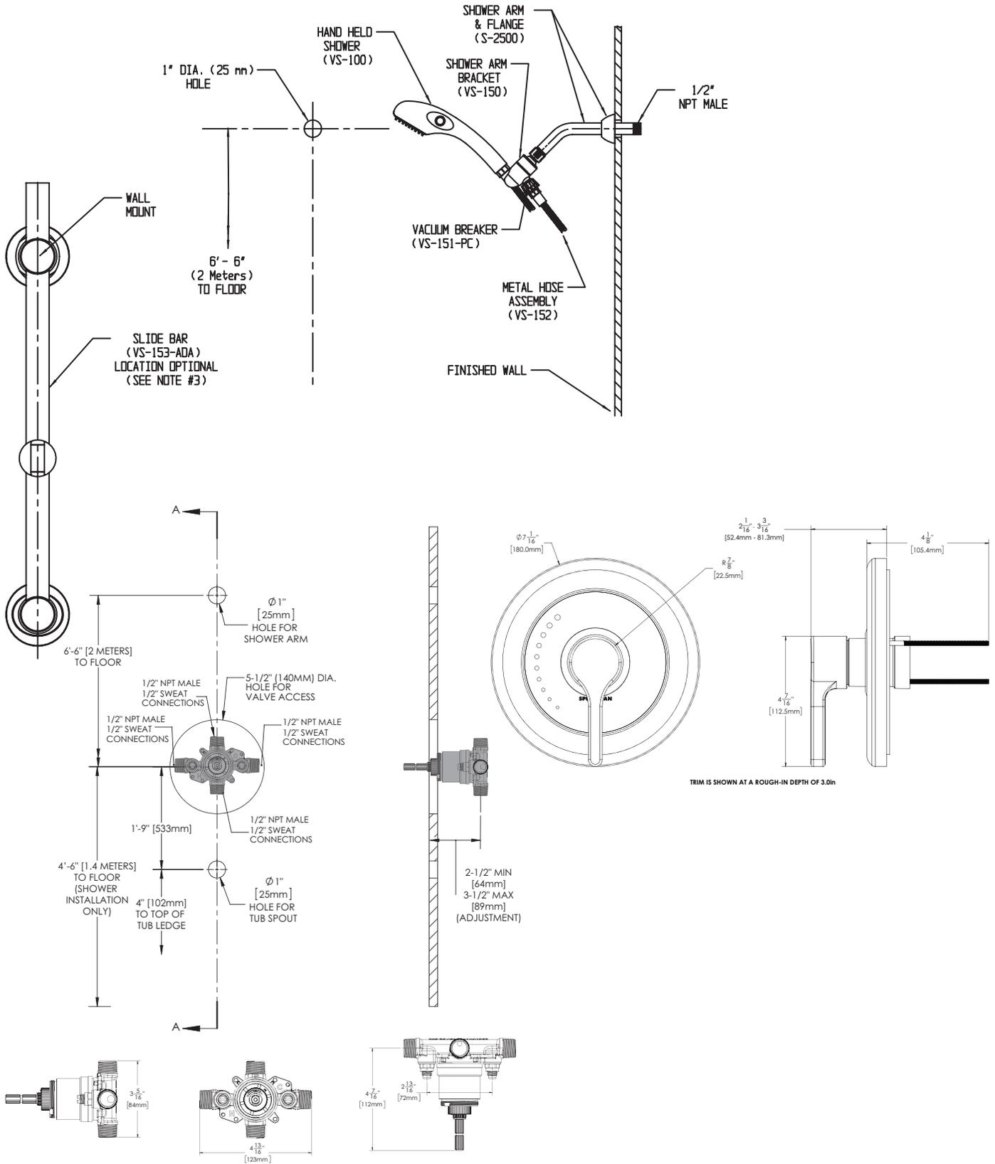
NOTE: 1. All dimensions are in inches (millimeters) unless otherwise specified and are subject to change without notice. 2. Unless otherwise specified, all inlets and outlets are 1/2" female copper sweat. 3. For ADA mounting locations, consult ADAAG, ANSI A117.1, or static regulations
